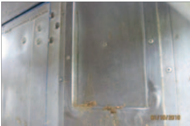
Water system used for bovines. Trough is closed by a moveable flap, which has to be pushed by the animals themselves in order to drink. Difficult to use for animals unaccustomed to this system since they cannot see the water. Inadequate, but commonly used in Long Distance Transports OCTOBER 2010
