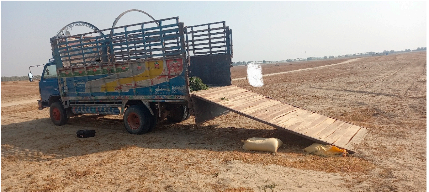
Figure 5. A truck fitted with a handmade modified ramp was used for the training. Since no special vehicle designed to transport camels was found in the study area, a normal truck was fitted with a handmade ramp.
